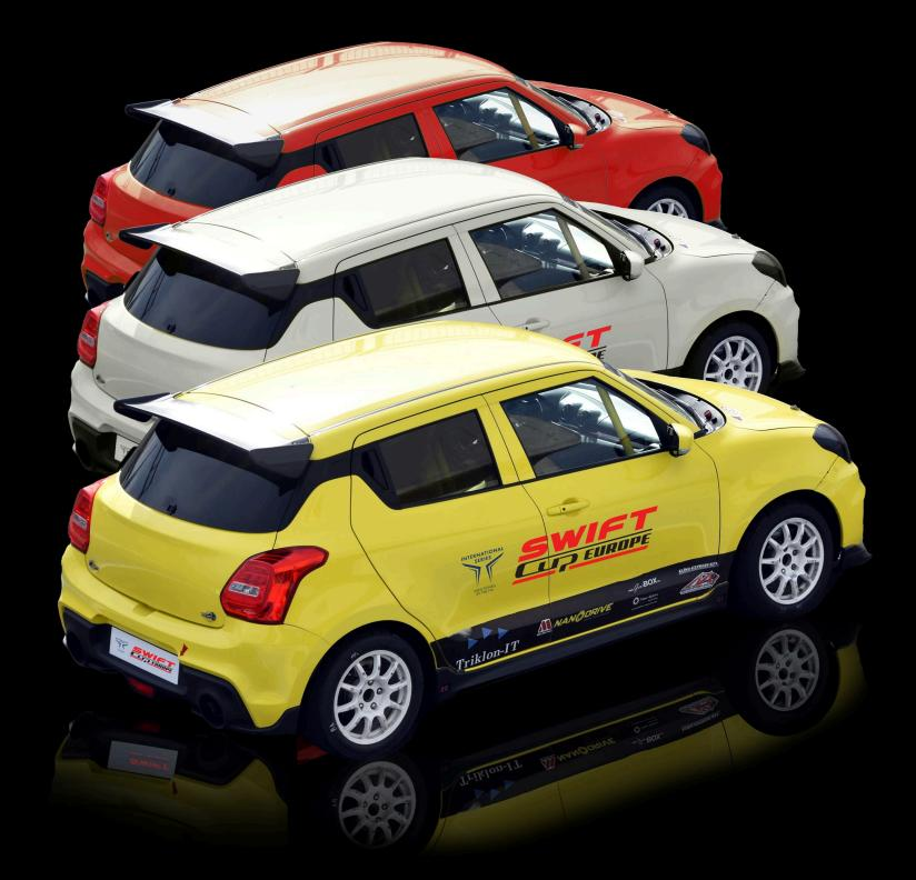
Minimal weight (without driver): 920 kg Yokohama semi-slick tyres 195/50R15 **Braid 7x15 ET36 rims** Öhlins dampers **AIM Solo Telemetry Tarox brakes**
